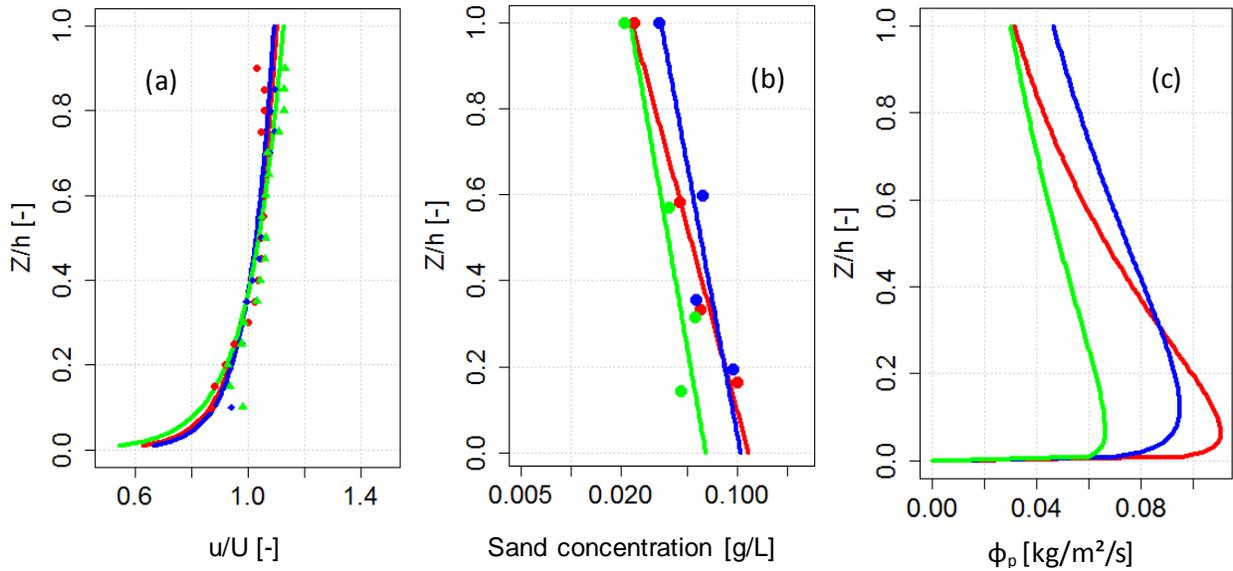
**Figure 7:** "Physically based method" applied to the Rhône River dataset (2018/01/22) (a) fitted ADCP velocities, (b) exponential profile (semi log scale), (c) Flux profile. Colors represent verticals numbers according to **Figure 4**.
