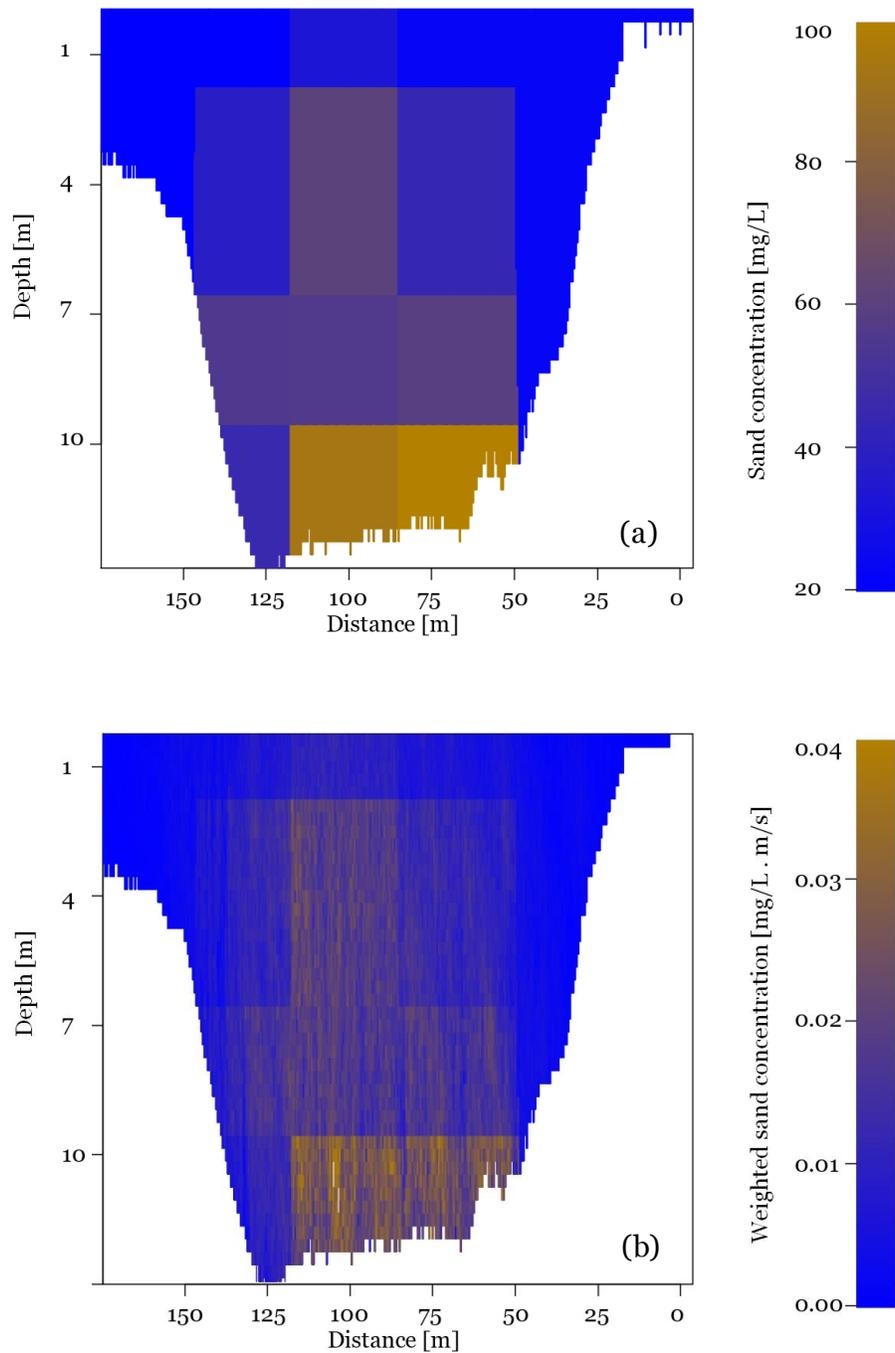
**Figure 6:** The nearest-neighbor method applied to individual point samples in the Rhône River at Lyon: (a) Sand concentration assigned to sub-sections according to the sample positions and ADCP data; (b) Velocity weighted sand concentration calculated for each ADCP cell.
