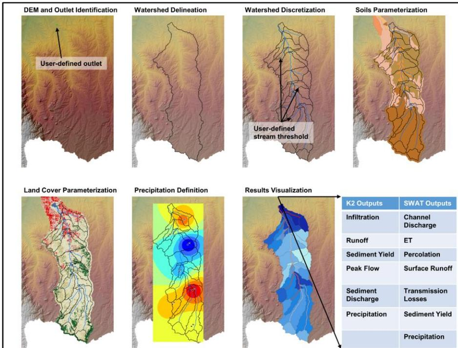
**Figure 1.** The required steps in AGWA to perform a watershed assessment. A DEM is used to delineate the watershed and subdivide it into model elements (i.e. hillslopes and channels for K2 and subwatersheds and channels for SWAT). The model elements are parameterized based on the DEM, soils, and land cover layers. The precipitation input is then selected from various sources. After the model is executed, the results are imported and visualized in the GIS.
