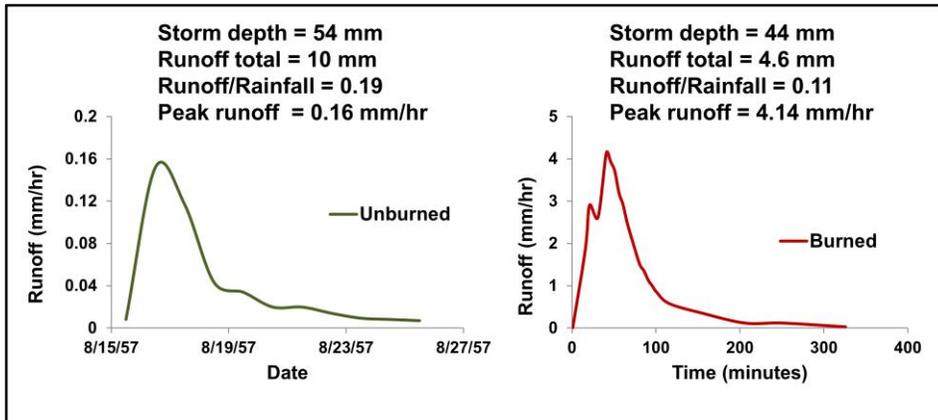
**Figure 2.** Pre-fire and Post-fire hydrographs recorded at Marshall Gulch, Arizona. This figure illustrates the difference in storm response for unburned and burned conditions (from Canfield et al. 2005, Scott 2016).
