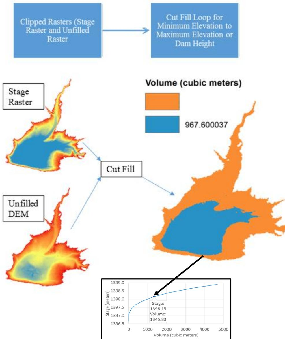
**Figure 3.** Cut-Fill function is part of a loop that calculates surface area and volume for pond stage from minimum elevation to maximum elevation. The final result is the stage-volume curve for the pond.
