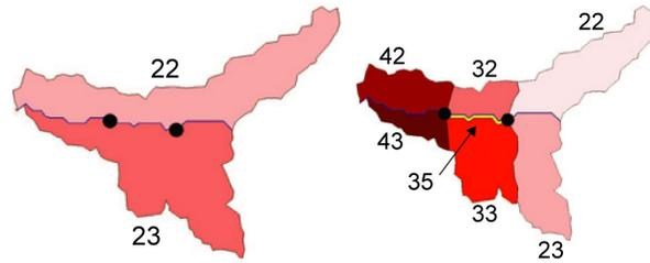
**Figure 4.** KINEROS2 Buffer discretization. (left) The unbuffered overland flow elements with buffer location and length defined by points. (right) The buffered overland elements (Goodrich et al. 2006)
