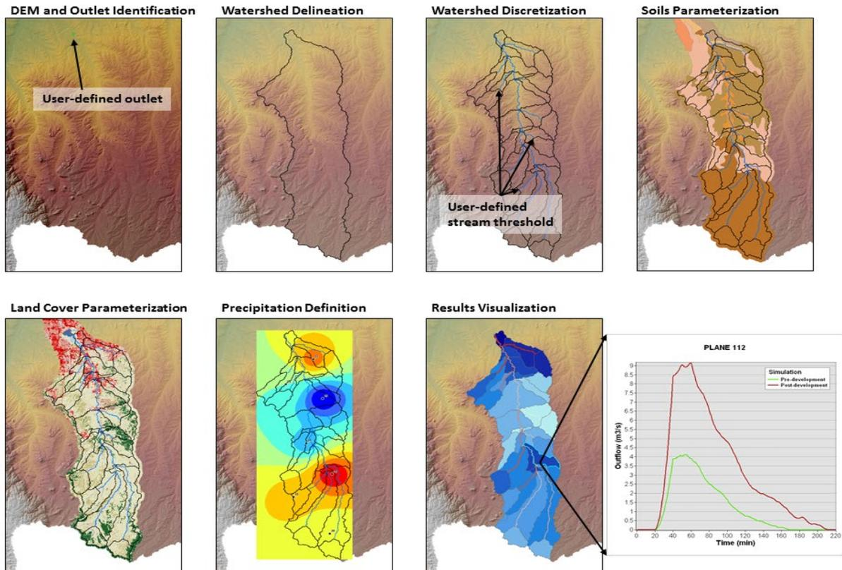
**Figure 2.** Primary steps in a watershed assessment using AGWA. Watershed delineation and subdivision into model elements is done using a DEM. Model elements are parameterized with soils, topography and land cover layers. Precipitation drives the model and spatially distributed results for each model element are imported and visualized in the GIS. Hydrographs and sedigraphs for any model element selected can also be displayed (lower right) (Goodrich et al. 2015).
