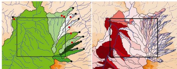
**Figure 3.** (left) Area of Interest outlet identification and delineation for the boundary. Red points indicate a potential outlet; black points are final watershed outlets that ensure watershed coverage of the area of interest. (right) Area of Interest watershed discretization
