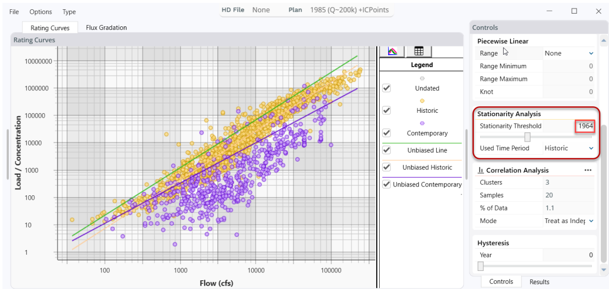
Figure 4. Arkansas River data at Tulsa stratified by pre-1964 (●) and post-1964 (●) samples, illustrating the non-stationarity of these data. The Rating Curve tool develops separate unbiased regressions for each time period.
