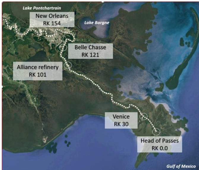
Figure 2: Map of the LMR channel (white dashed line) and the location of key infrastructure susceptible to damage from saltwater intrusion relative to Head of Passes measured by river kilometer (RK).
