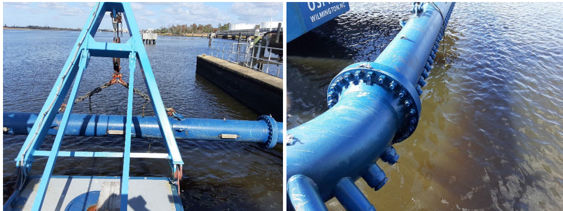
Figure 1. The jet bar on a water injection dredge used by the port of North Carolina.
