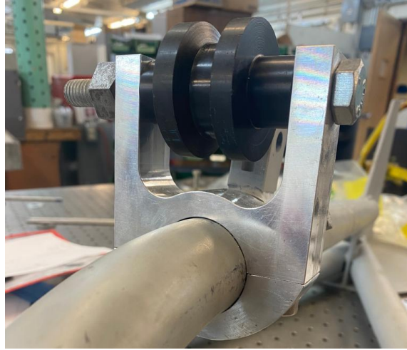
Figure 16. Fabricated Top-Tube Mounted Pulley
