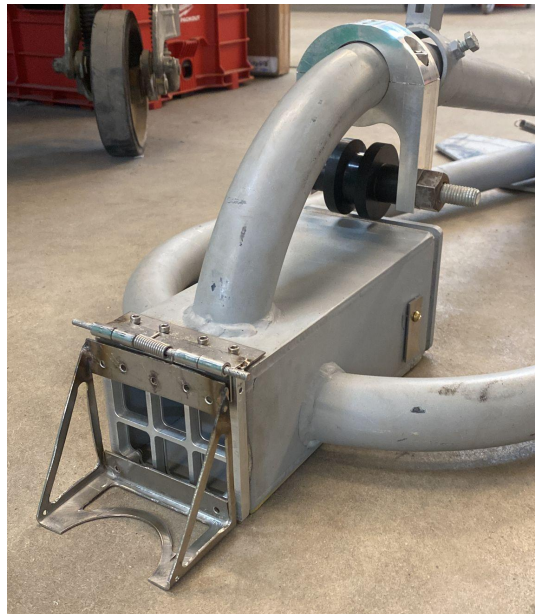
Figure 17. Fabricated Top-Tube Mounted Attachment
