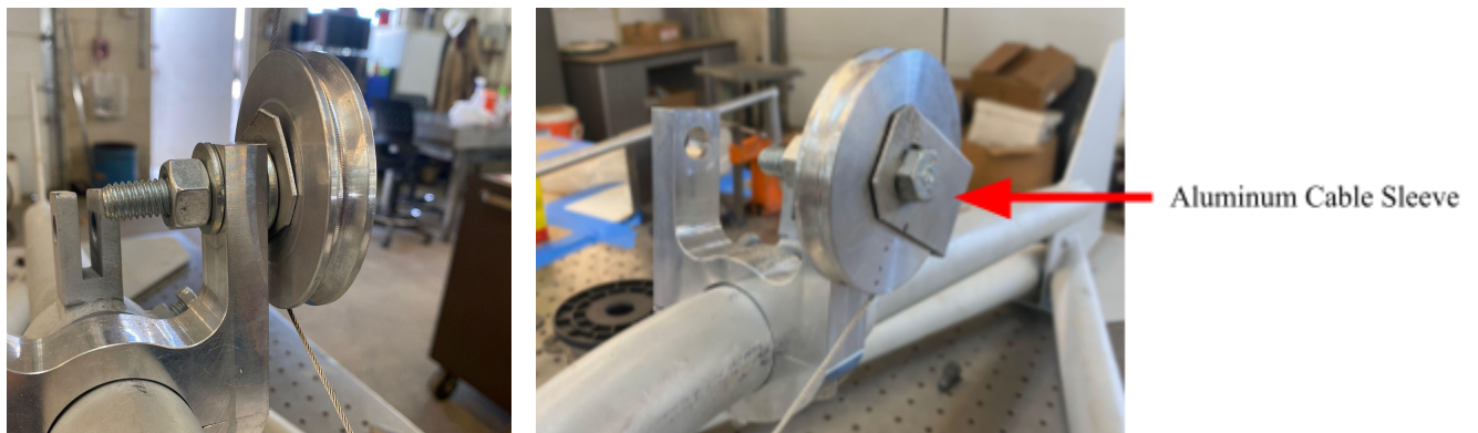
Figure 26. Final Design - Modified Tube Mounted Pulley
