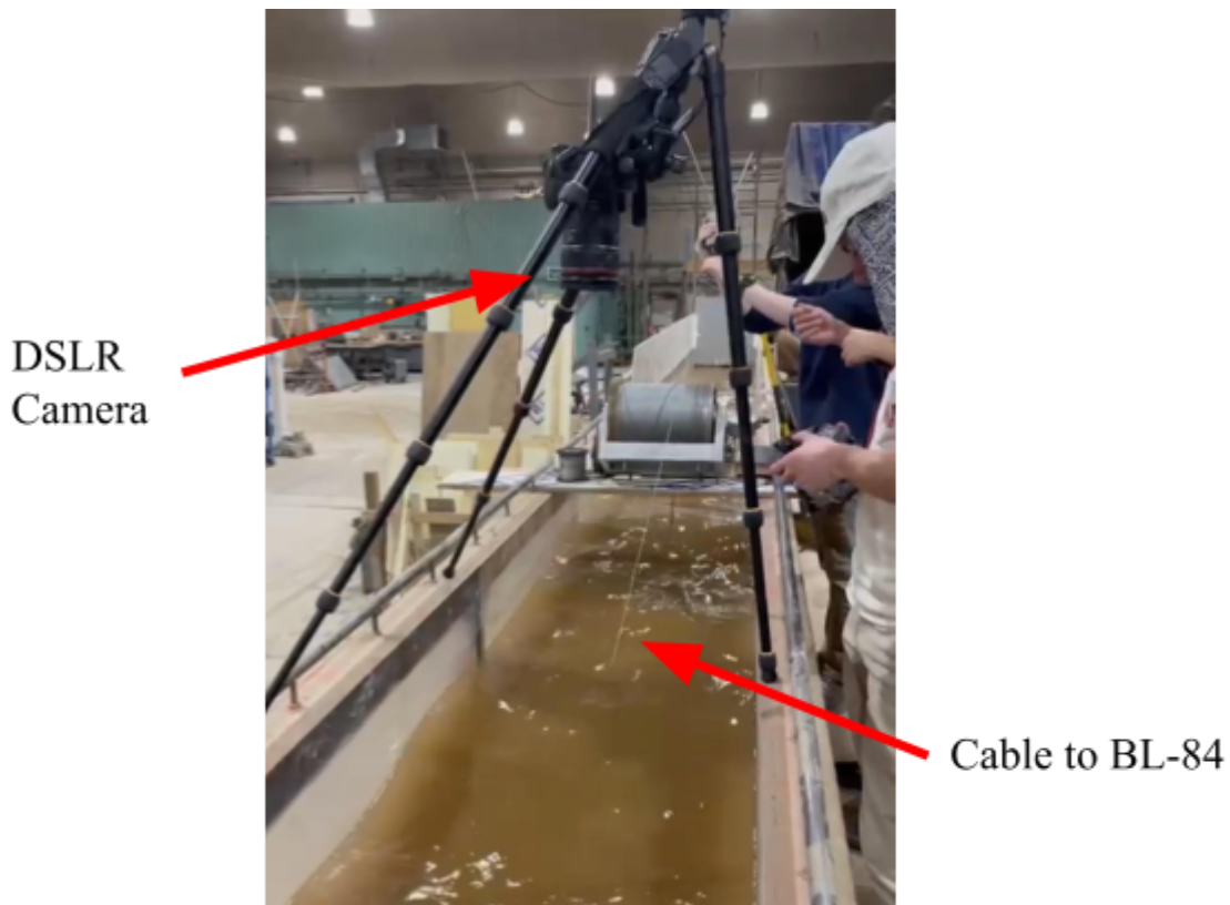
Figure 41 : DSLR camera setup on flume
