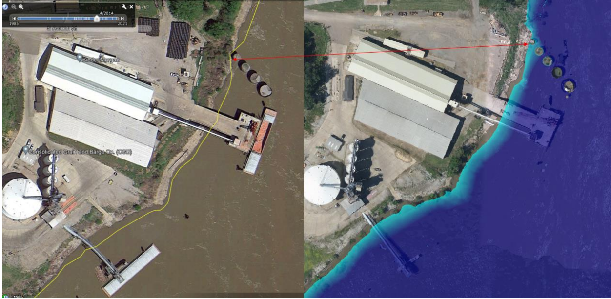
Figure 3. Google image on April 22, 2015, with flow of 1,000,000 cfs compared to HEC-RAS 2D model result with flow at 1,000,000 cfs.
