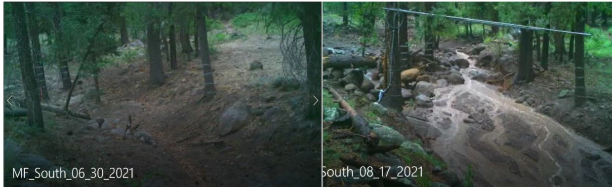
Figure 10. Channel configuration at Museum South in June 2021 and August 2021, note the change in channel geometry. Channel geometry changed drastically after each storm, some with net scour and others with net aggradation, making stage-discharge determinations challenging.
