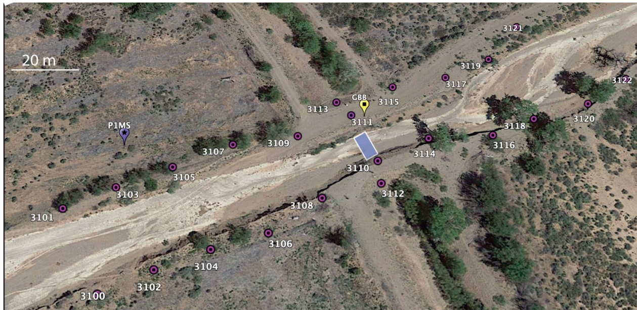
Figure 5 Location of the in-channel sediment monitoring research station (blue rectangle) and distribution of the seismic stations deployed during 2021 along the channel. Purple circles are seismic nodes; P1MS and GBB are broadband stations. (Courtesy S. Bilek)
