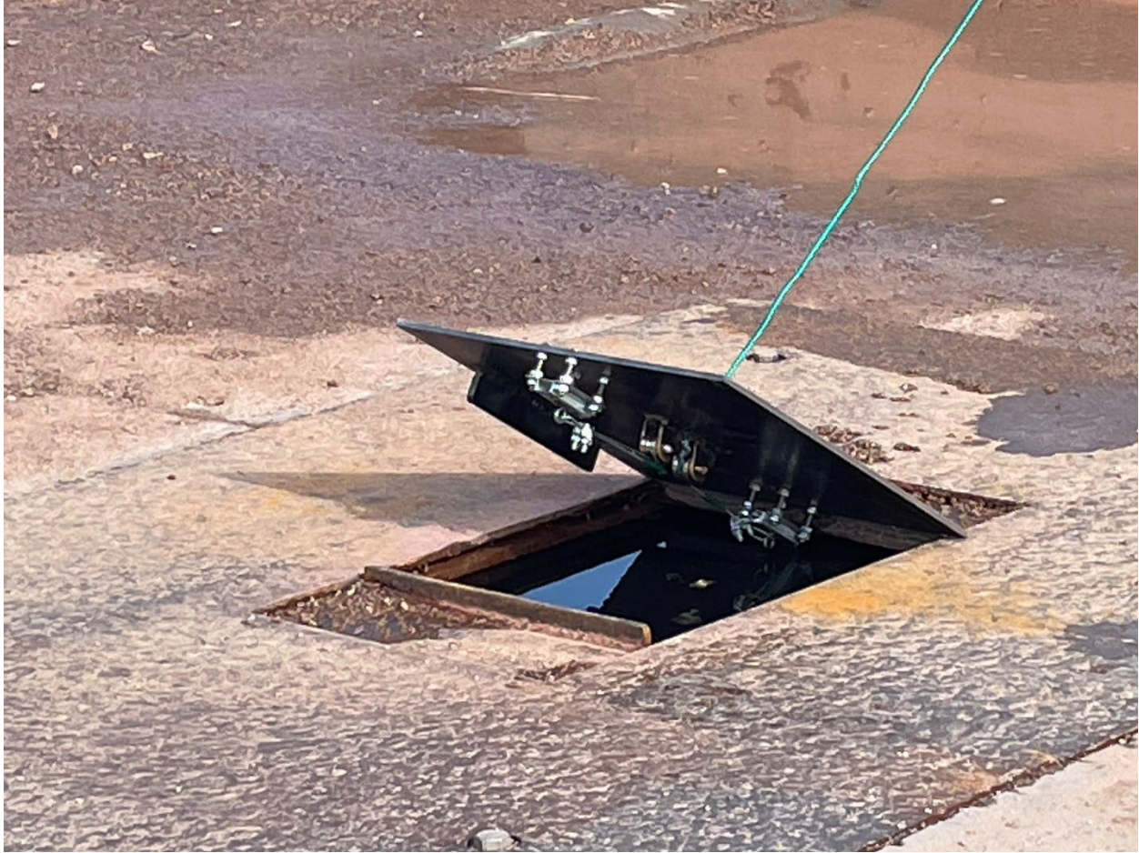
Figure 4. Lid covering the right slot sampler so that selective bedload sampling can occur during the peak of a storm event
