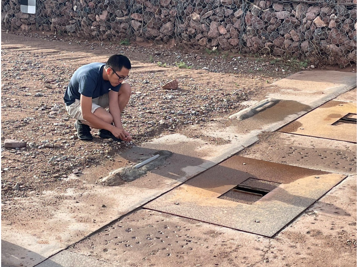
Figure 3. Graduate student Loc Luong testing center pipe microphone after installation, replacing the previously-deployed plate microphone
