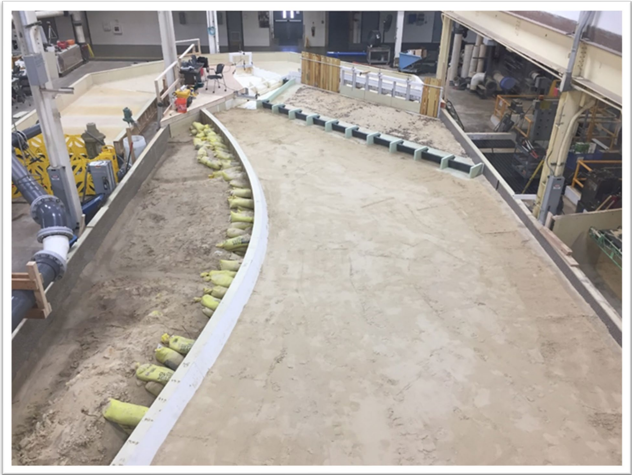
Figure 6. Graded bed of scaled sand prior to the start of a mobile bed test
