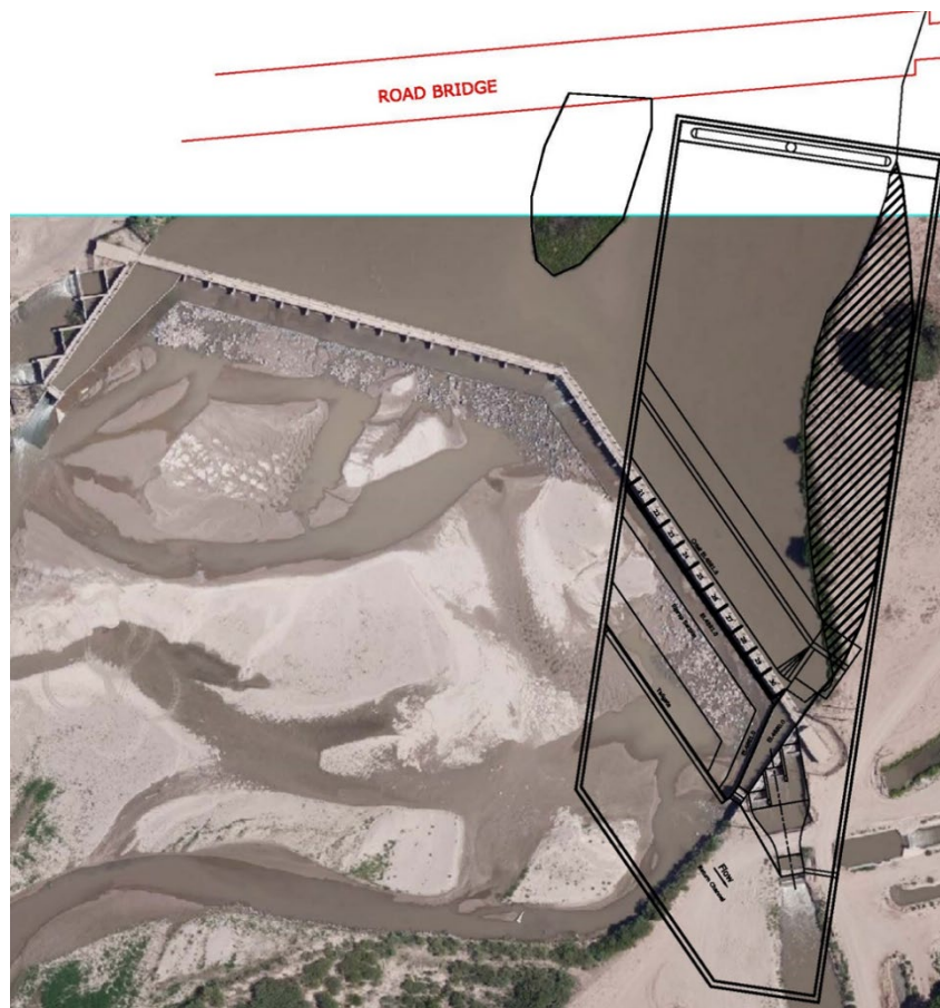
Figure 4. Aerial overlay showing extents of the 1:8 scale physical model covering a portion of the Rio Grande, IDD and Peralta headworks. The hatched area shows the east bank removal for realignment as part of the Options that were physically modeled.
