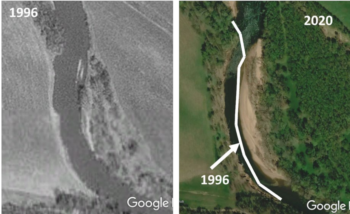
Figure 9. Riverbank erosion at bank 2 between 1996 and 2020; flow from bottom
