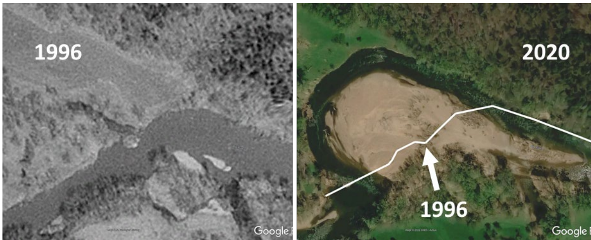
Figure 7. Riverbank erosion at bank 1 between 1996 and 2020; flow from right
