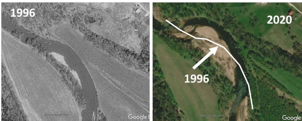
Figure 11. Riverbank erosion at bank 3 between 1996 and 2020; flow from bottom
