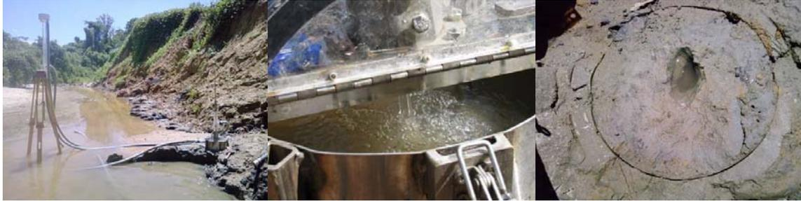
Figure 4. View of the a) jet test device setup, b) jet of water applied on the streambank material, and c) scour generated on the streambank material after a test
